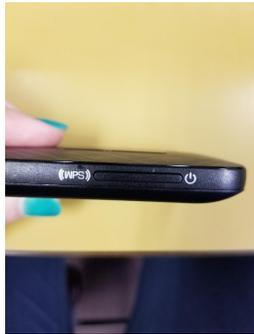
Turn on hotspot by holding down the long, thin power button on the side of the device until the lights flash on
